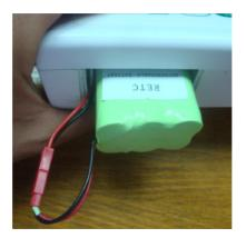
4. Push the battery pack into the battery holder then locate the cable connector above the battery pack.
