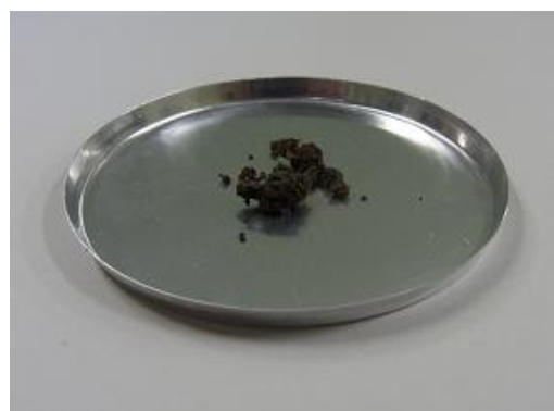
Volume reduced due to drying
